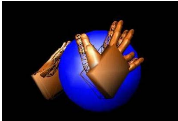
Figure 1: Holding a Ball with Two Virtual Hands; the Opaque Hands Show the Positions of the Virtual Hands, the Wireframe Hands Show the Positions of the User's Real Hands. They are, in contrast to the virtual hands, able to penetrate the ball.
